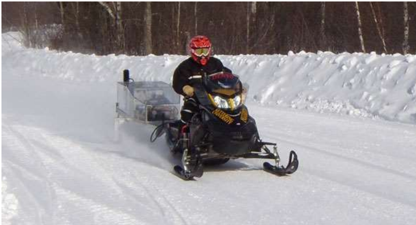
Figure 1. In-Service emissions analyzer being pulled by competition snowmobile
