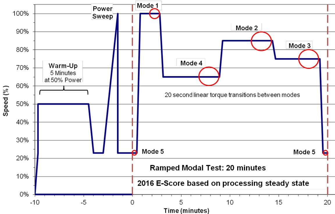
Power Sweep determines Max. Power. Speed and Torque for each mode defined by 5-mode
