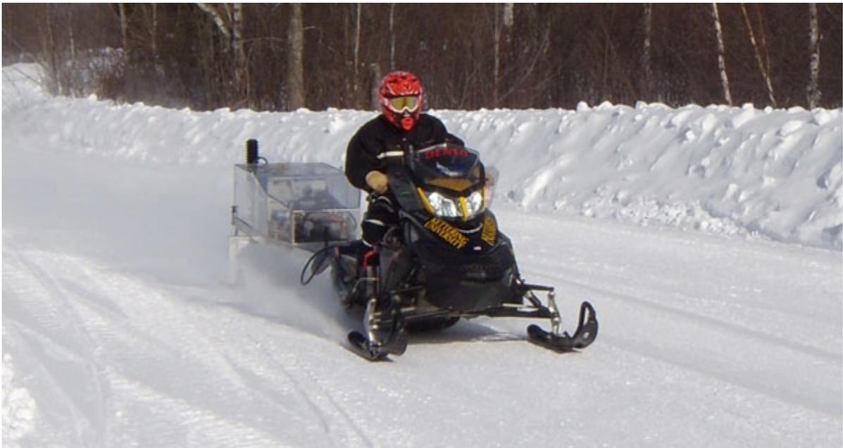
Figure 1. In-Service emissions analyzer being pulled by competition snowmobile
